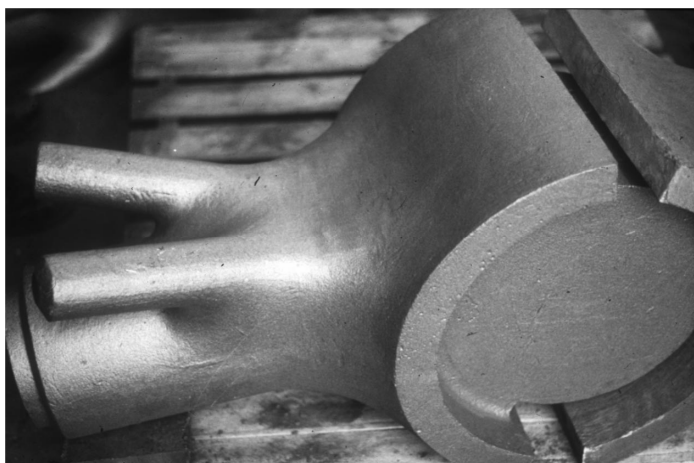
Figure 11. Weldable cast steel node for the hinge at the crown of the primary trusses
