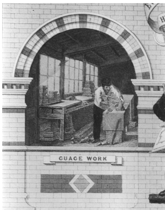
Figure 7 Large brick axe lies against the chopping block in A.J. Waudby's 1863 depiction of a cutting shed, (The People's History Museum, Manchester)
