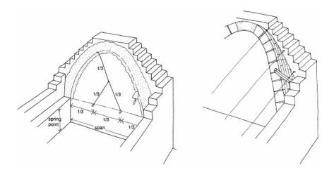
Figure 7. Phases construction of vault
