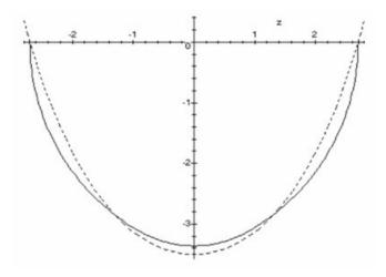
Figure 9. Polycentric curve (continuous) and catenary function (hidden)
