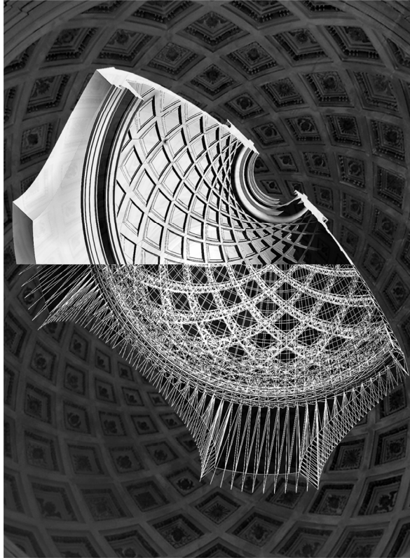
Figure 5. Three-dimensional computer model of the Anet dome: analysis of the geometric-construction process (G. Fallacara 2005)
