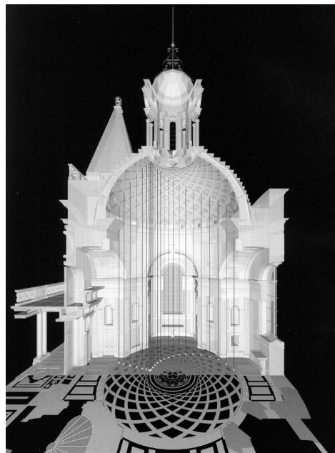
Figure 7. Perspective section of the chapel at Anet: projective correspondence between the design of the mouldings and that of the pavement below (Gava and Trintinaglia 2004, fig.33)
