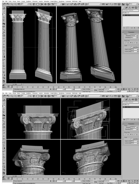
Figure 7. Skew transformations: Composite columns according to de l'Orme's idea.
