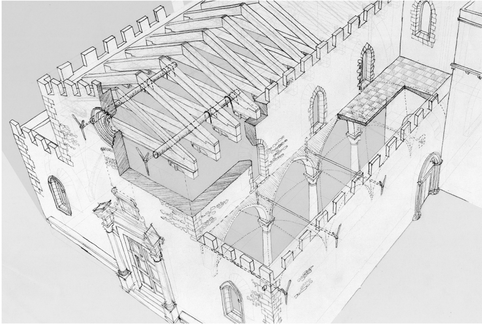
Figure 10. Drawing of St. Nicholas, Taormina. The tie-rods were inserted after the great earthquake of 1693.
