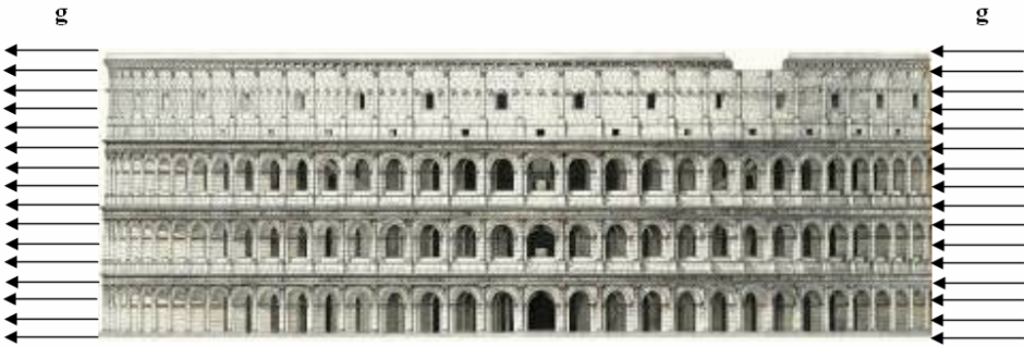
Figure 9 The plan of the Coliseum and the direction of the seismic action
