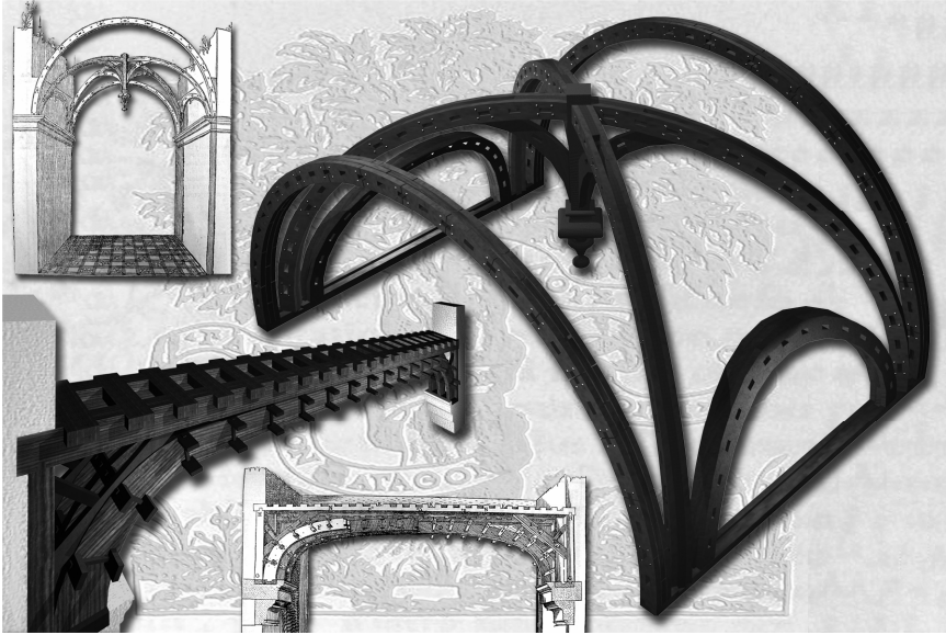
Figure 5. De l'Orme's roofs and floors.
