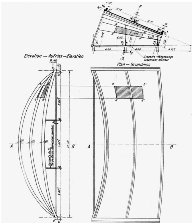
Figure 3. Design of the roof 17.00 m span, built by Entreprises Limousin and tested by Fauconnier for the Cie Métropolitain de Paris (Fauconnier 1934, fig. 2).
