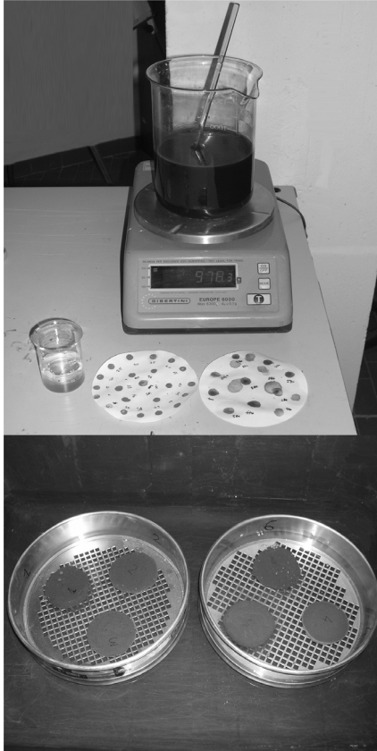
Figure 4. Methylene blue test measures the earth reactivity, while soaking test is to determine resistance to water immersion. In this way it is possible to verify the effectiveness of different earth stabilisers.
