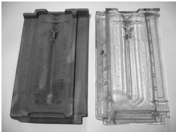
Figure 9. Marseille clay roof tile and Saint-Gobain glass roof tile used in the roof of surveyed dwelling.
