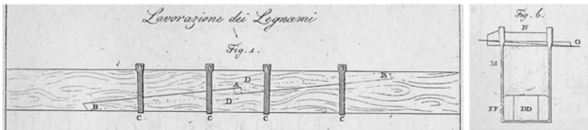
Figure 7: Possible use of U-shaped straps illustrated in Valadier’s treatise.. On the right, the mentioned wooden element (“ stacciola ”) to be inserted between the beam and the strap (DD)
