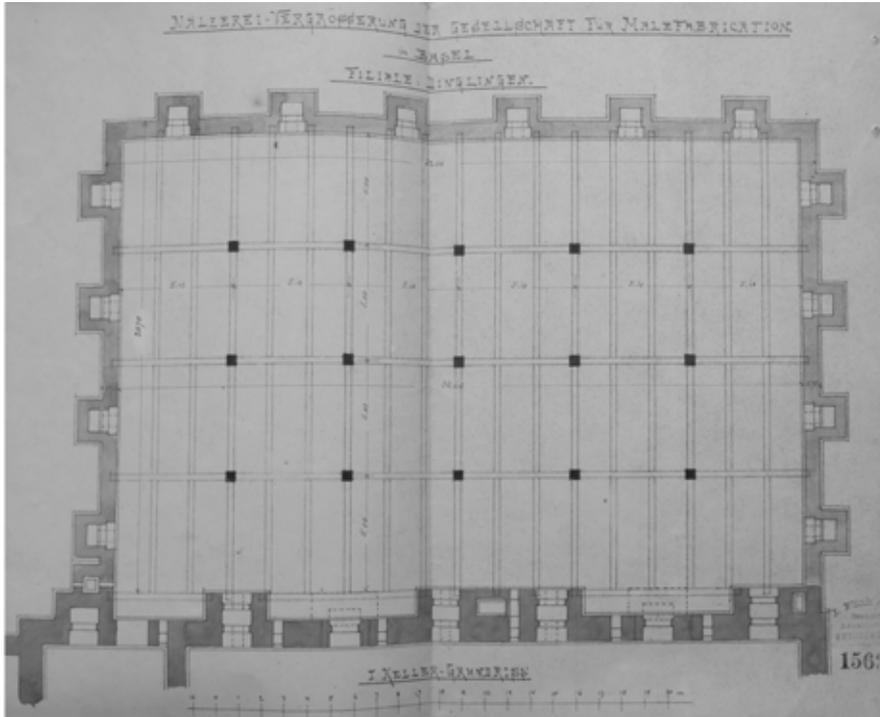
Figure 6: Ground floor plan, with the 15 columns highlighted as part of the application of building permission, 1895. Photo: Kuban. Lahr Building Authority Archive.
