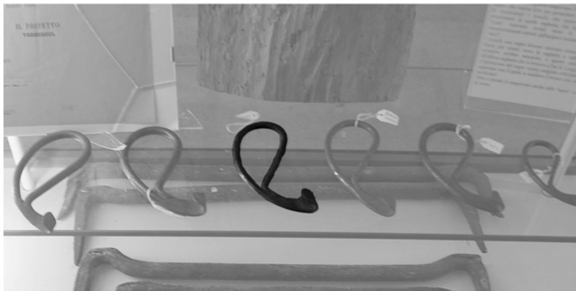
Fig. 4 Traditional tool to imprint marks on timber in the Rafting Museum in Codissago (picture: author).
